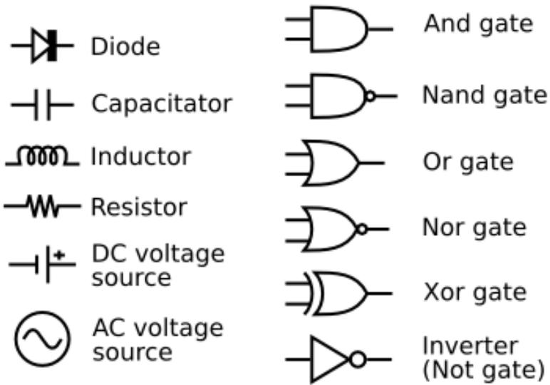
These symbols show some of the common circuit elements. A diode only lets current flow one way (the direction of the arrow). A resistor slows down the flow of current.
