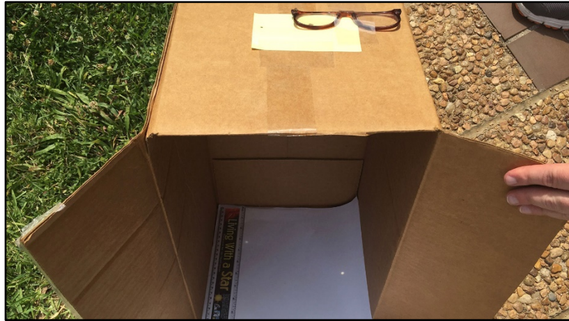
Figure 7 A large, opened box on its side with a pinhole on the top surface allows viewers to see the projected Sun's image inside. Courtesy, Rice Space Institute, https://space.rice.edu/eclipse/safe_eclipse_observing.html
