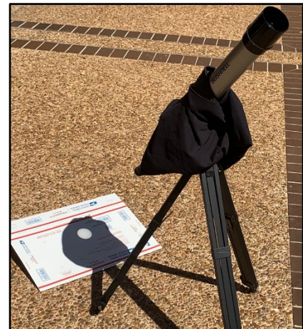
Figure 9 A refracting telescope with a dark cloth projects the Sun's image
