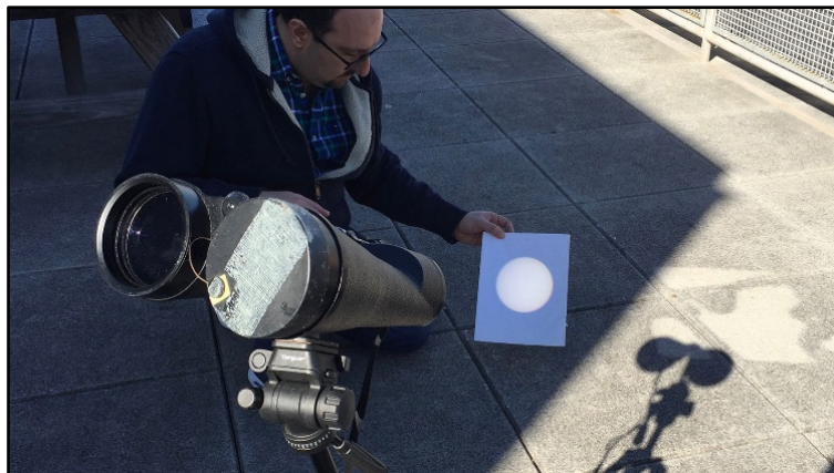
Figure 9 A refracting telescope with a dark cloth projects the Sun's image
