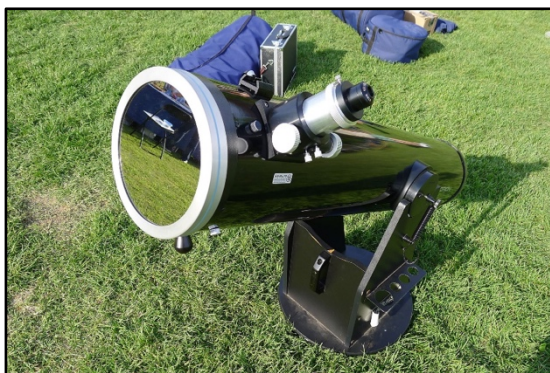
Figure 11 An image of a reflecting telescope with a solar filter attached over the objective lens. Courtesy, NASA, credited to Carolyn Slivinski https://solarsystem.nasa.gov/eclipses/safety/#:~:text=When%20watching%20a%20partial%20or,safe%20for%20viewing%20the%20Sun.
