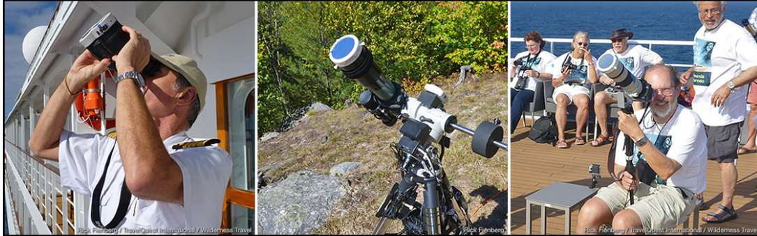
Figure 12 Three pictures showing solar filters correctly attached. Left-a pair of binoculars held by a man; middle-a telescope mounted on a tripod; right- a telescope held by a man. All three pictures show how the solar filters are placed over the objective lenses. Courtesy, AAS https://eclipse.aas.org/eye-safety/optics-filters
