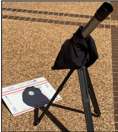
Figure 11 A refracting telescope with a dark cloth projects the Sun's image onto white paper on the ground. Courtesy, Rice Space Institute https://space.rice.edu/eclipse/safe_eclipse_observing.html
