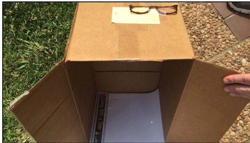
Figure 10 A large, opened box on its side with a pinhole on the top surface allows viewers to see the projected Sun's image inside. Courtesy, Rice Space Institute, https://space.rice.edu/eclipse/safe_eclipse_observing.html
