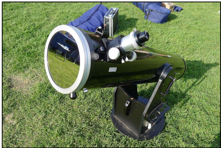
Figure 14 An image of a reflecting telescope with a solar filter attached over the objective lens. Courtesy, NASA, credited to Carolyn Slivinski https://solarsystem.nasa.gov/eclipses/safety/#:~:text=When%20watching%20a%20partial%20or, safe%20for%20viewing%20the%20Sun.
