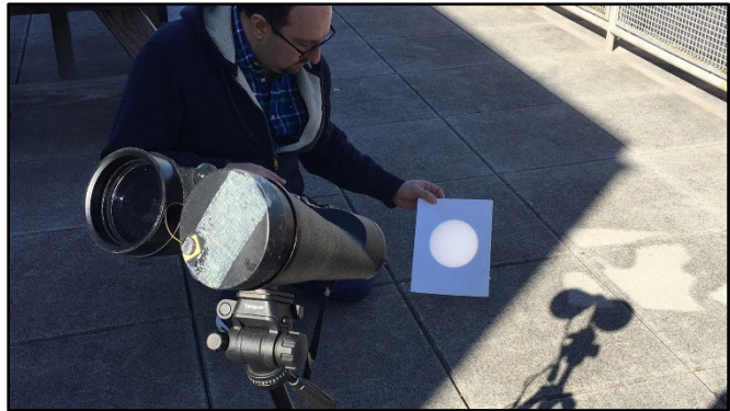
Figure 12 Binoculars with one lens covered and the other allowing the Sun's image to be cast onto a white sheet of paper on the ground. Courtesy, Rice Space Institute https://space.rice.edu/eclipse/safe_eclipse_observing.html
